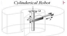
Fig 2: Cylindrical configuration [5]
